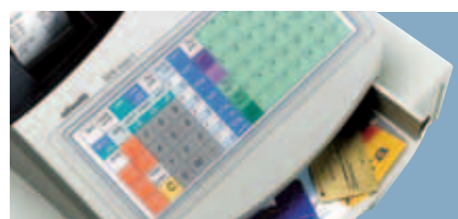
Customizable keyboard, with 42 PLU keys and direct selection of up to 126 articles
